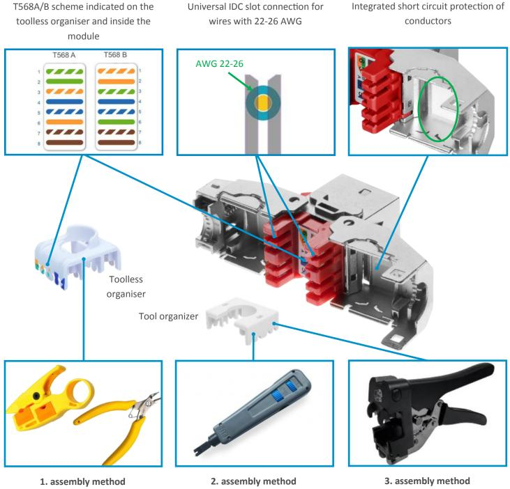
Tool: using 110 IDC impact tool
